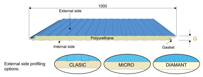
Upon request, there can be produced thermo-insulated panels of polyisocyanurate (PIR) foam, with fire resistance.
