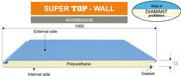
Self-supporting steel insulated panel from polyurethane cu with hidden fixing – architectural model, which due to their anchorage method provide exquisite aesthetics and reliability. The articulation of this type of panel provides the possibility of both vertical as well as horizontal installation.
